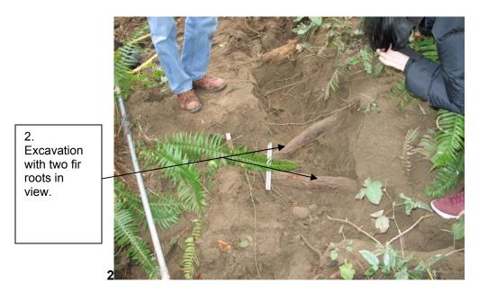
The soil exposed by the excavation was sandy loam. A small lens of silt clay was also encountered. I was able to insert my probe another 36" from the bottom of the excavation without much force, indicating that the sandy well drained soils continue in this area. Given the soil conditions on the site it would not surprise me to find more roots of significant size growing at a greater depth than was exposed during this investigation.
